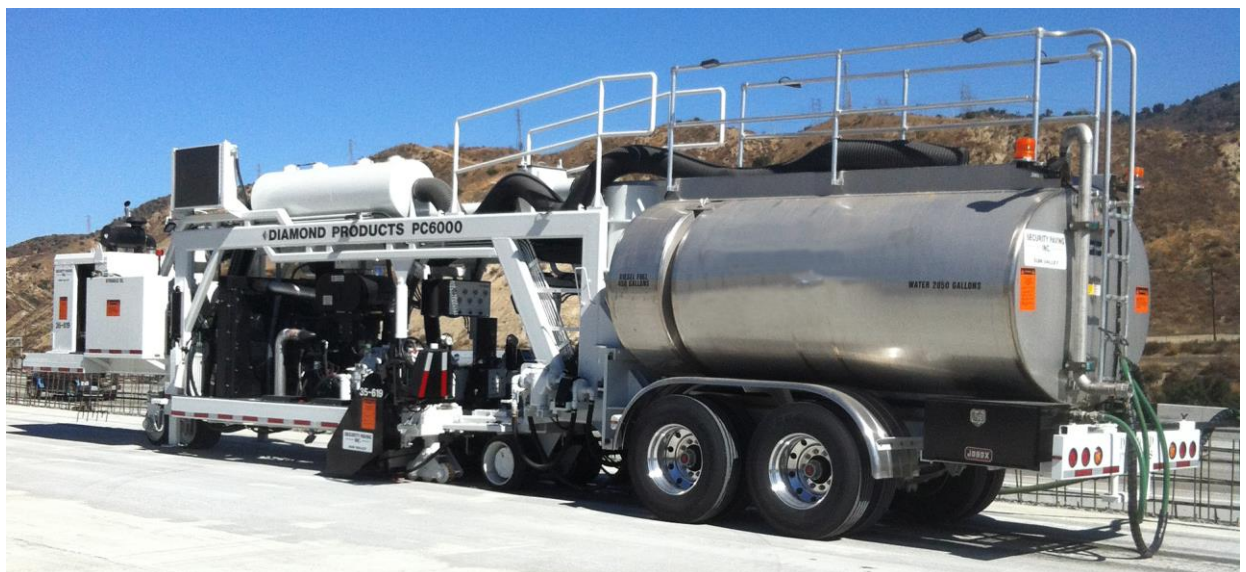
DIAMOND GRINDING PLANT
